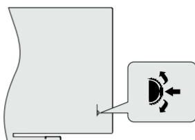
The control switch allows you to control the Programme and Quick Standby-On functions of the TV.
